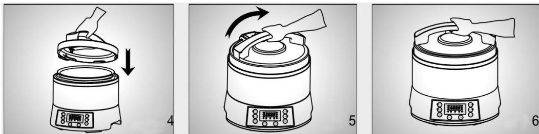
6. Adjust the Pressure Limiting Valve to the “Airtight” position and ensure that the Float Valve sinks.
