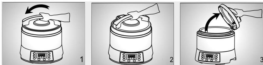
1. **How to open the lid:** When the lid of the cooker is at the closed position, hold the Handle and turn it counter-clockwise until you reach the Opened-Lid position, Lift up and the lid will swing open vertically.
