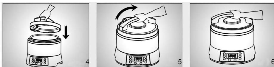
2. **How to close the lid:** When the Lid of the cooker is in vertical position, hold the handle and close it downwards at the Opened Lid position. Turn clockwise until you reach the Closed Lid position.
