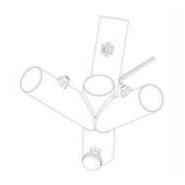
Whilst holding the leg / post coupling upside down, take a wooden leg and insert the flat end into one of the leg tubes and push down all the way as shown below. Using the Allen key, tighten the grub screw until it is firm and holding the wooden leg in place
