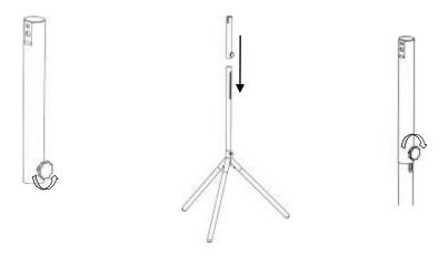
Turn the height adjustment knob clockwise so that the screw thread is located inside the slot.
